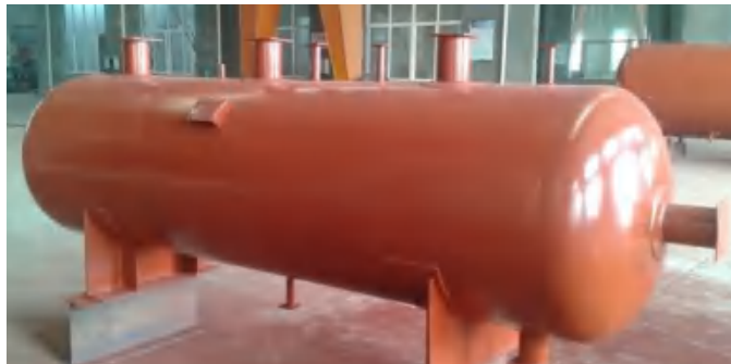
Fig. 1 Heat storage tank adopting phase change heat storage technology
